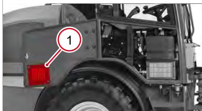
III. 192: Kabinens ventilationsfilter
